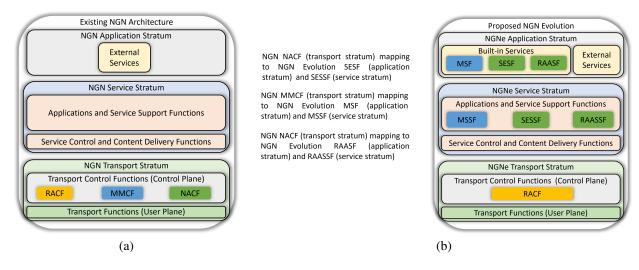
Fig. 1. (a) Existing NGN Architecture (b) Proposed Architecture for NGN Evolution
