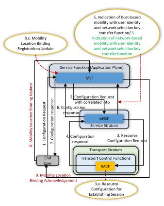
Fig. 3. Information flow for host-based/network-based mobility service
